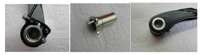
• Once disassembled use 220-250 grit sand paper on the leading edge of the bushing pivot bolt to smooth the first 3-5mm:
